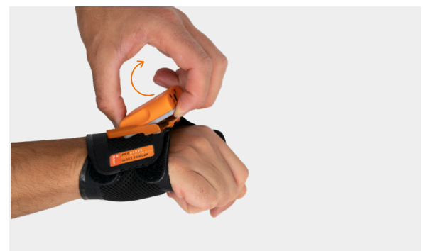
Use the fingers to press between scanner and the fastening rail of the Index Trigger. Press scanner up slightly and push it forward without scratching over the pins.
